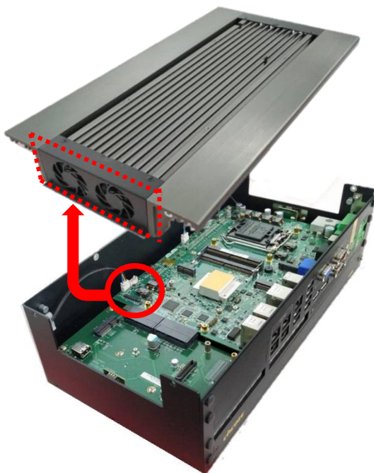
POWER1 (FAN OUT Control)
