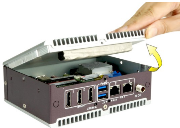
Figure 3-2: Bottom Surface Removal
