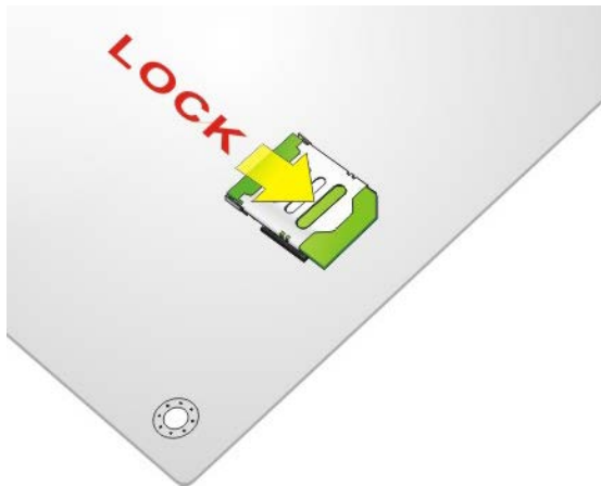
Figure 4-14: Lock SIM Card Slot Cover
