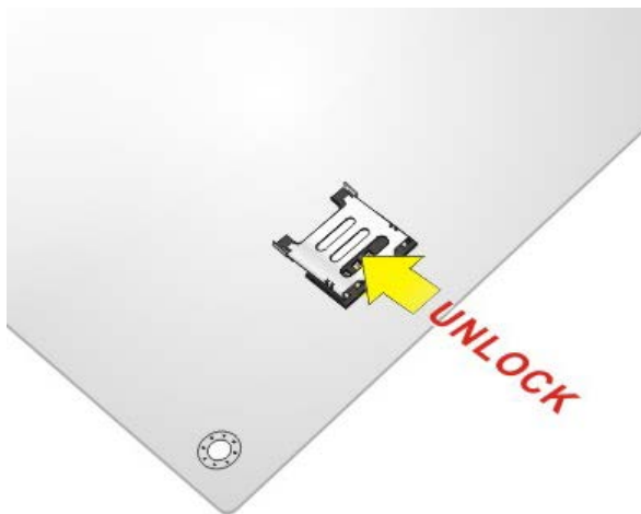
Figure 4-12: Unlock SIM Card Slot Cover
