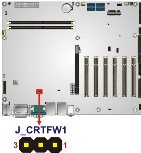
Figure 3-7: CRT FW Update Connector Location
