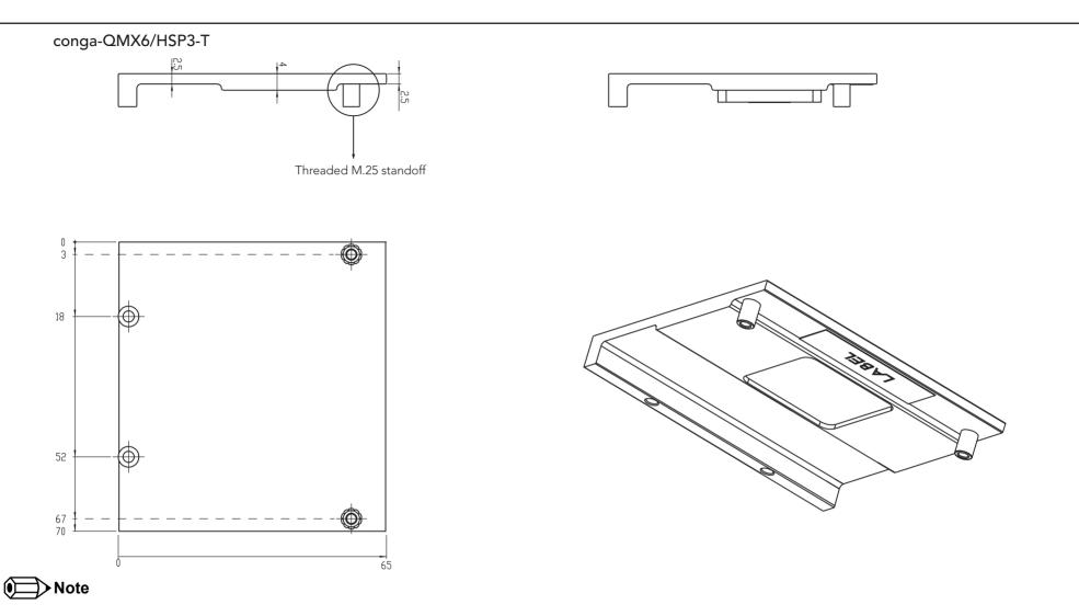
All measurements are in millimeters. Torque specification for heatspreader screws is 0.3 Nm. Mechanical system assembly mounting shall follow the valid DIN/ISO specifications.
