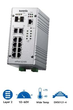
Korenix JetNet 5210G, the DIN-Rail type Industrial Gigabit Managed Switch is designed with eight 10/100TX ports and two Gigabit RJ-45 / SFP combo ports. The two Gigabit Ethernet combo ports provide high speed uplink to connect with higher level backbone switches with Korenix MSR<sup>™</sup> network redundancy technology, while ensuring the reliability of data transfer through the exclusive recovery time in several milliseconds and seamless restoration.
