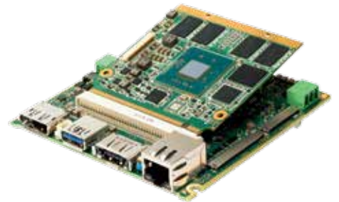
Fig 1. Computer-on-Module concept, carrier board and computer module
