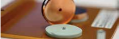
Pin avoids sliding of the copper block
