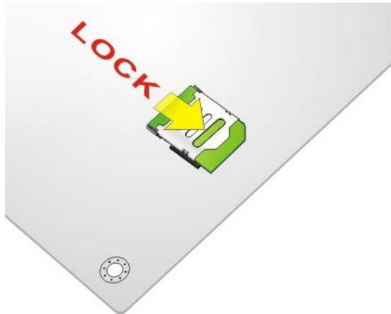
Figure 4-7: Lock SIM Card Slot Cover
