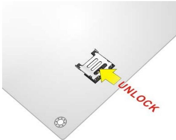
**Figure 4-5: Unlock SIM Card Slot Cover**
