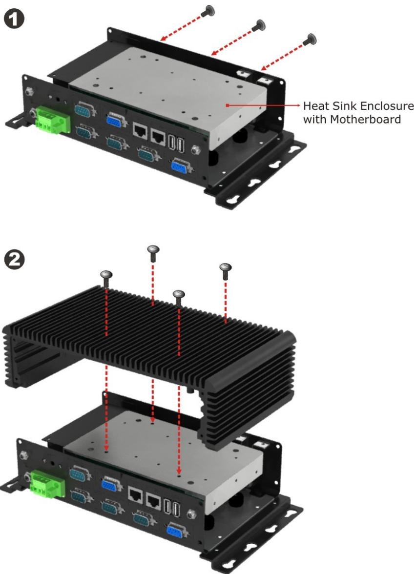
Figure 4-16: Motherboard Installation Example
