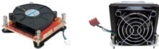
Figure 4-5: Cooling Kits (CF-1156A-RS and CF-1156E-RS)
