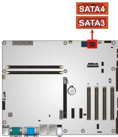
Figure 3-25: SATA 3Gb/s Drive Connector Locations
