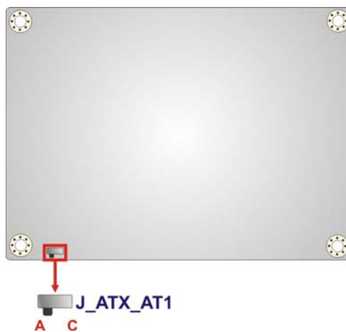
Figure 3-2: AT/ATX Mode Select Switch Location
