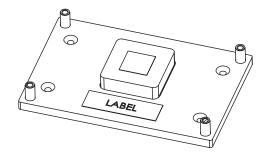
M2.5x11mm threaded standoff for threaded version or Ø2.7x11mm nonthreaded standoff for borehole version
