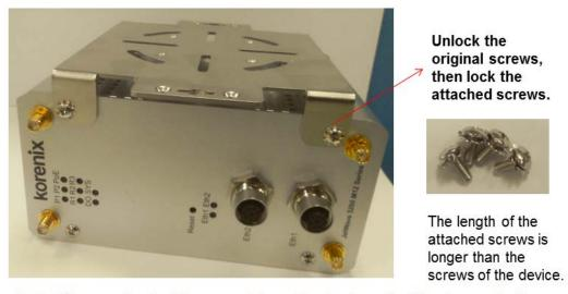
**Note:** Please notice that the screw hole on the front panel will be damaged after lock/unlock few times. DO NOT often change the celling mounting kit!
