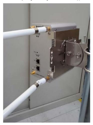
4. In some cases, you may need to install the celling mount plate first then lock the AP/Gateway to the celling-mount plate.
