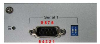
Pin 1: DCD Pin 2: RXD Pin 3: TXD
