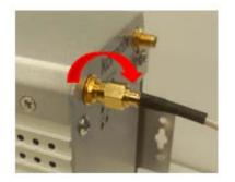
Use the same way to lock the attached WIFI antennas, it is clockwise direction as well. **Note** that the counter-clockwise direction will loosen the antenna immediately.
