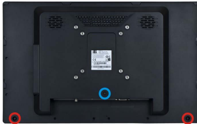
Figure 3-3: AFL3-W15A-BT Back Cover Retention Screws
