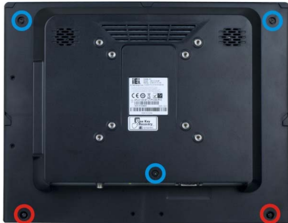
Figure 3-2: AFL3-12A-BT Back Cover Retention Screws
