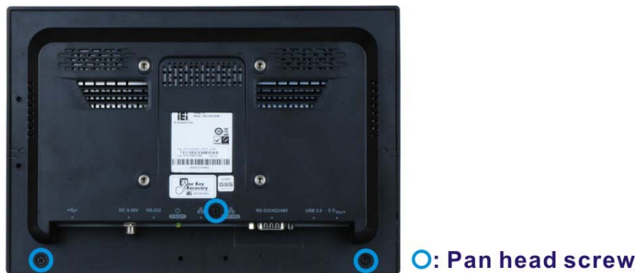
Figure 3-1: AFL3-W10A-BT Back Cover Retention Screws
