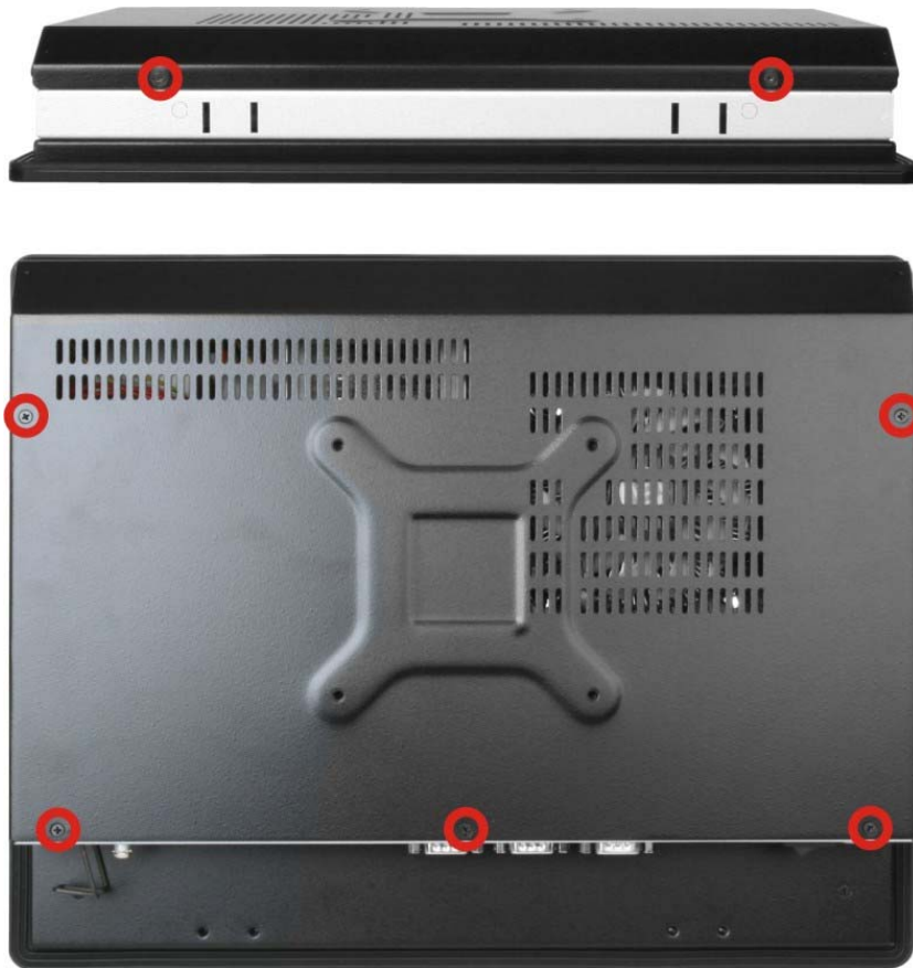
Figure 3-1: PPC-F15A-H81 Back Cover Retention Screws
