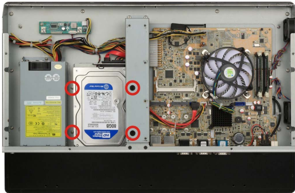
Figure 3-11: Replacing the PPC-F22A/F24A-H81 HDD Bracket
