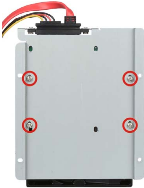
Figure 3-10: 3.5" HDD Retention Screws
