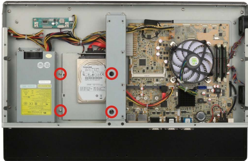
Figure 3-8: Replacing the PPC-F22A/F24A-H81 HDD Bracket
