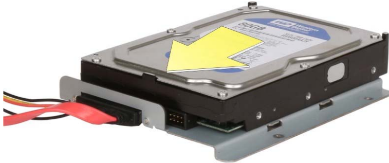
Figure 3-9: Connecting the Hard Drive to the HDD Bracket
