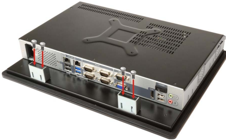
Figure 3-22: PPC-F15A-H81 Mounting Bracket Installation
