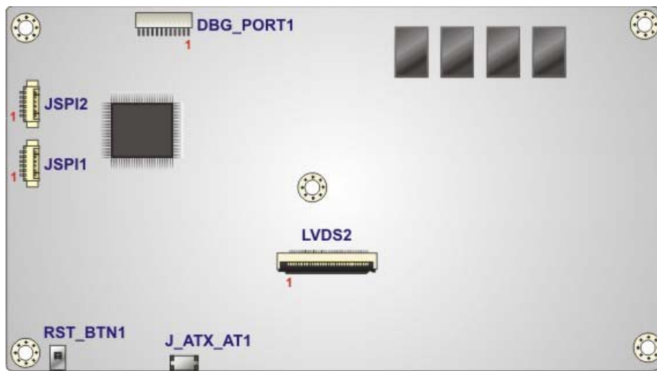
Figure 6-2: Main Board Layout Diagram (Solder Side)
