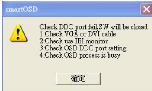
Figure C-18: DDC Port Failure
