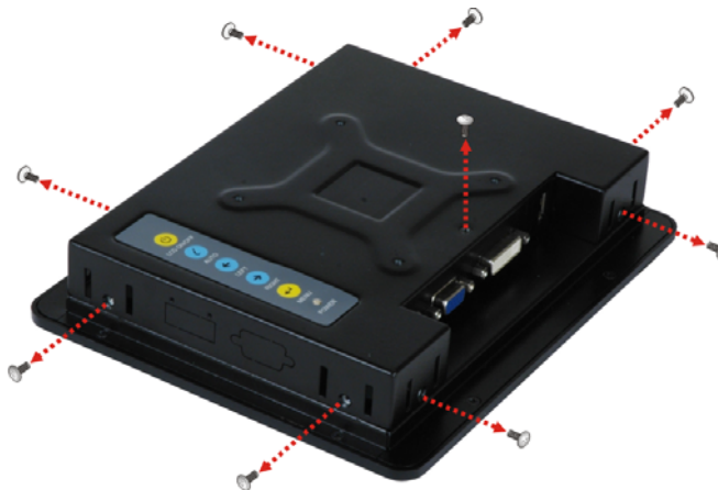
Figure 3-9: Rear Panel Retention Screw Removal (6.5" & 8")
