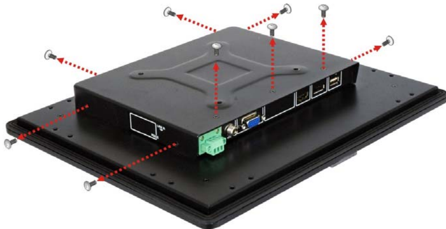
Figure 3-10: Rear Panel Retention Screw Removal (12" – 24")
