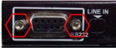
Figure 3-12: Hex Jack Screws for Securing RS-232 Connector
