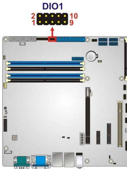
Figure 3-7: Digital I/O Connector Location
