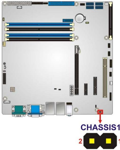
**Figure 3-4: Chassis Intrusion Connector Location**
