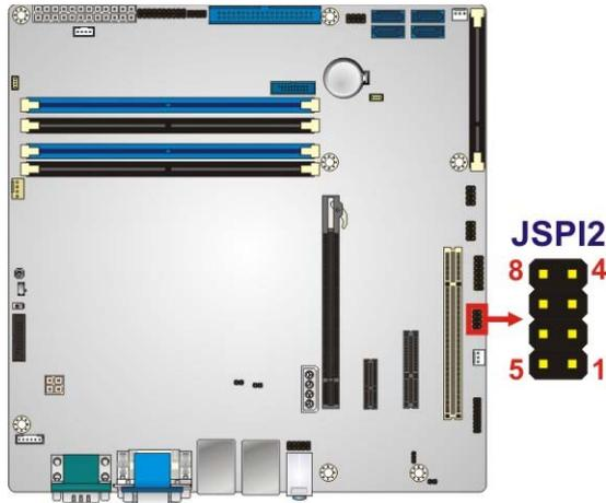
**Figure 3-24: SPI EC Flash Connector Location**
