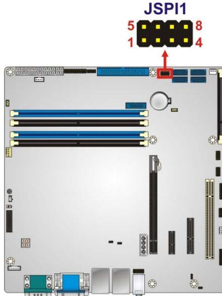
**Figure 3-23: SPI Flash Connector Location**
