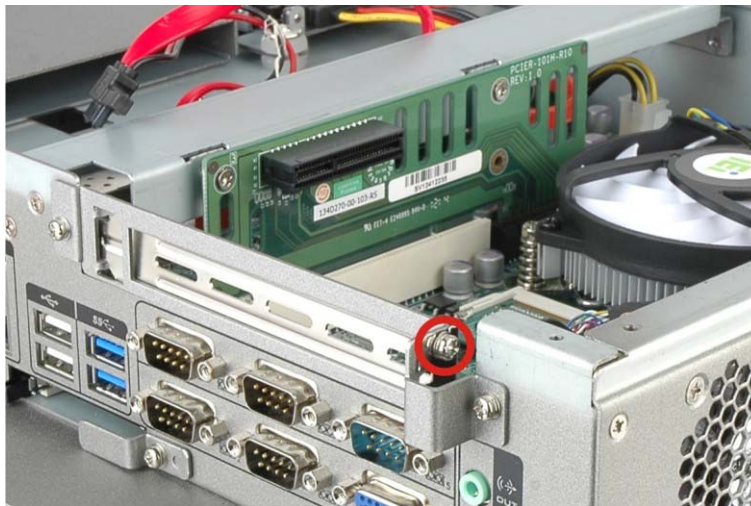
Figure 3-19: Expansion Slot Retention Screw
