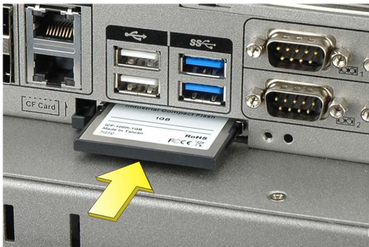
Figure 3-8: Installing the CompactFlash® Card
