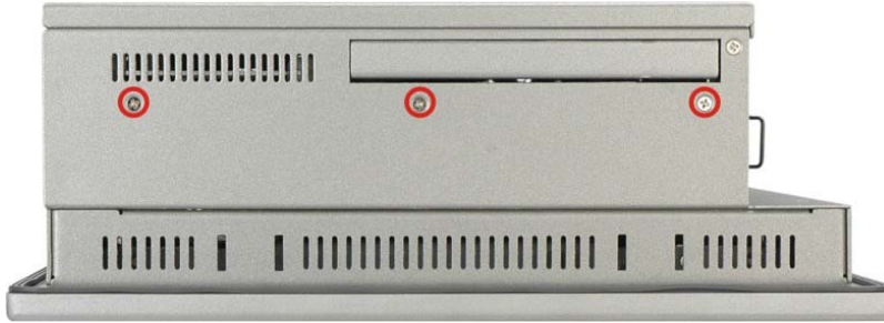
Figure 4-4: PPC-5150A-H61 Side Panel Elevated Platform Screws
