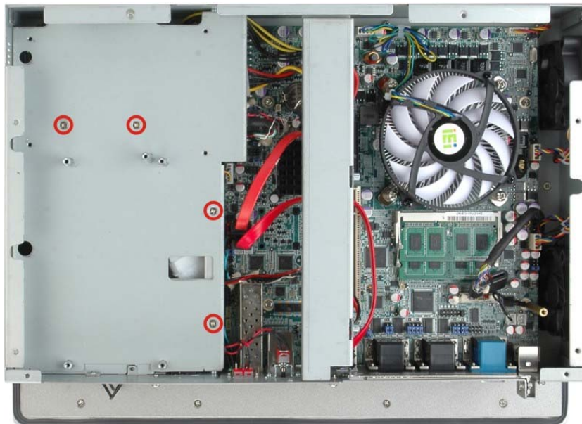
Figure 4-6: PPC-5150A-H61 Internal Elevated Platform Screws
