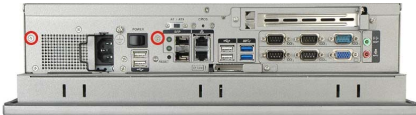
Figure 4-5: PPC-5150A-H61 Bottom Panel Elevated Platform Screws
