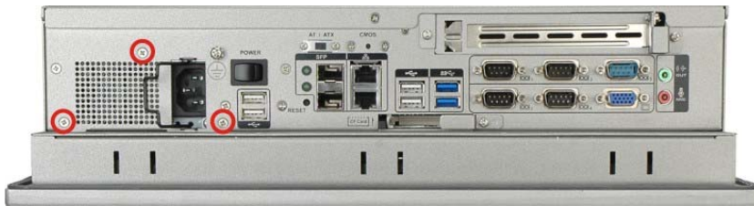
Figure 4-9: PSU Bottom Panel Screws
