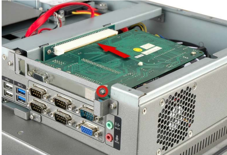
Figure 3-17: Installing the PCI Card
