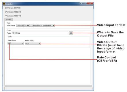
Step5. Repeat Step2 ~ Step4 to configure the connected input device.
