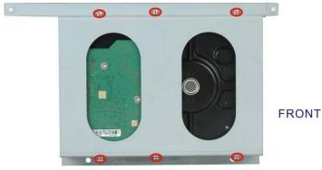
HDD retention screws
