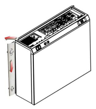
Figure 12: Wall-mounting the EBC-3000
