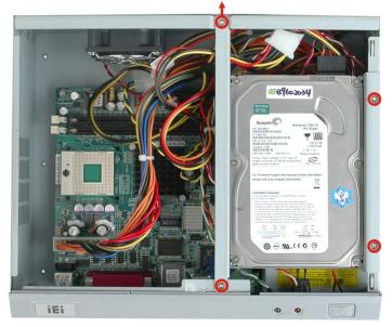
Figure 10: HDD/ODD Bracket Retention Screws
