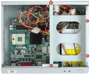
Figure 4: HDD Bracket Retention Screws
