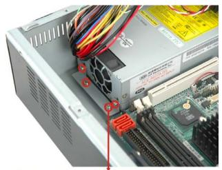
Power supply bracket retention screws
