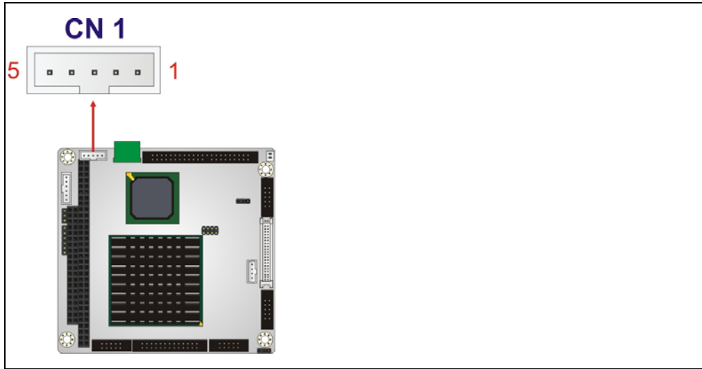
Figure 3-12: LCD Inverter Connector Location
