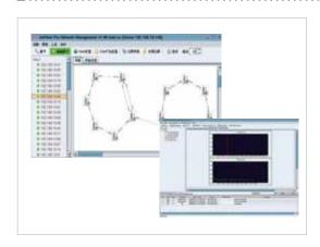
Korenix NMS periodically monitors and reports selected nodes and interface statistics to provide real-time status of the device availability as well as traffic performance in a timely basis. By incorporating SNMP gatherer function, users can review the gathered SNMP MIB data performance without a need of additional device.
