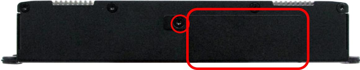
2. Turn over the module and loose 2 screws at the back of the connector cover.
