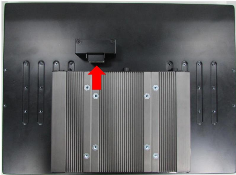
4. Have the studs screwed to the display module through the holes of the PC module.
