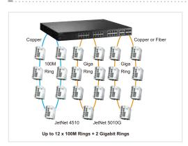
The JetNet 5728G-24P series supports the new generation ring technology – MSR<sup>TM</sup> which includes various new technologies for redundancy applications and structures of different networks. The PoE switch allows to aggregate up to 14 Rapid Super Rings, including 12 Fast Ethernet plus 2 gigabit Ethernet Rings. With the MSRTM technology, a node can be configured to multiple rings with the failover time in as little as 5ms, and zero-second of restoration time.
