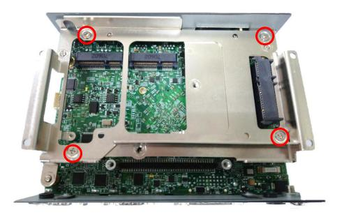
2. Make the PCB side of the HDD face up, place the HDD bracket on it. Ensure the direction of bracket is correct and use 3 provided screws to assemble HDD and HDD bracket together.
