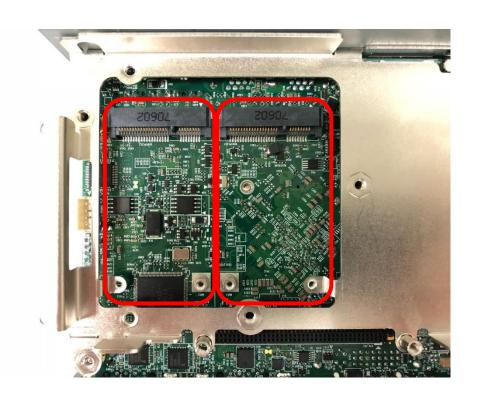
3. Tilt the Mini PCIe modules at 45 degree angle and insert it to the slot until the goldpated connector of module contacted firmly with the slot.
