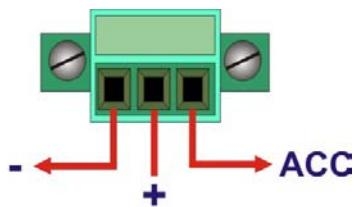
**Figure 3-16: 3-pin Terminal Block**
