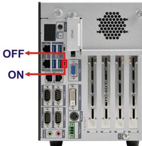
Figure 3-9: ACC Mode Switch
