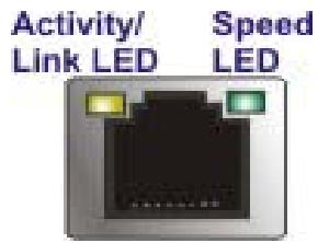
Figure 3-15: RJ-45 Ethernet Connector
