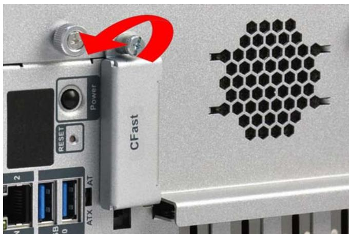
**Figure 3-1: CFast Socket**
