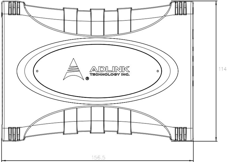
**Figure 1-3: USB-2401 Module Side View**
