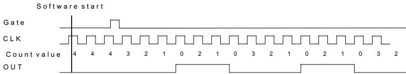
**Figure 3-17: Mode 7-Single-Triggered Continuous Pulse**
