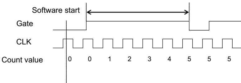
**Figure 3-13: Mode 3-Single Pulse-Width Measurement**
