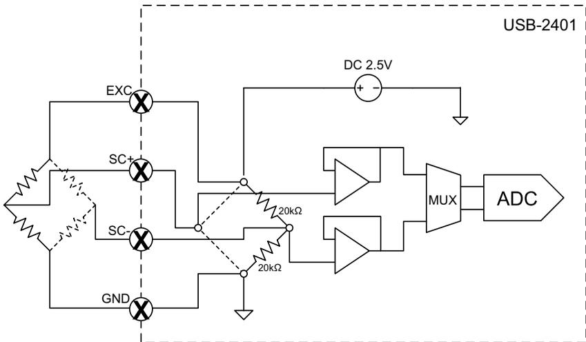
Figure 3-5: Full Bridge and Half Bridge Connection
