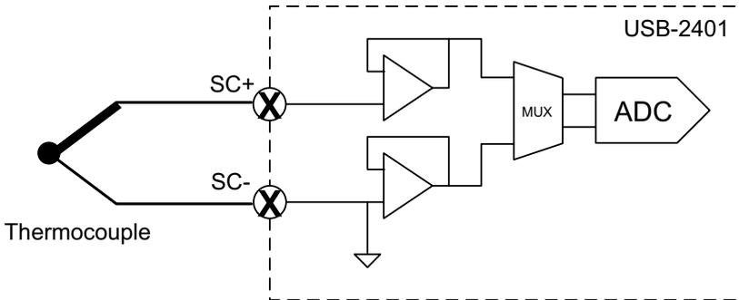
**Figure 3-6: Thermocouple Connection**
