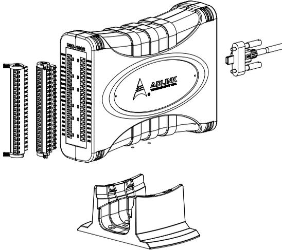
**Figure 1-5: Module, Stand, Connector, and USB Cable**
