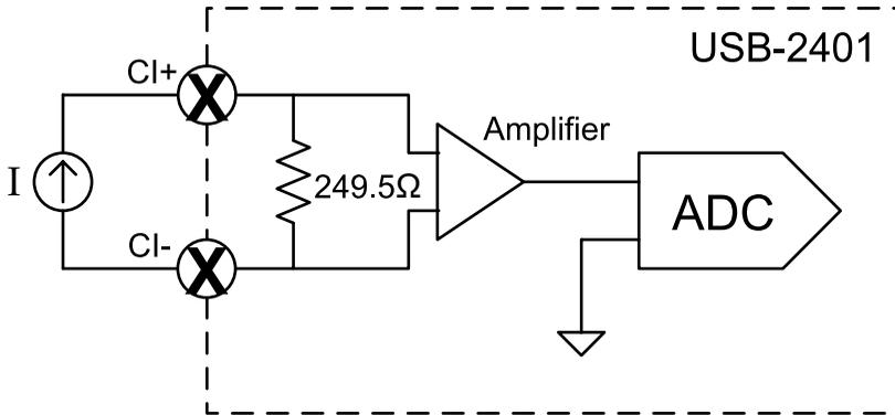
**Figure 3-4: Current Source Connection**
