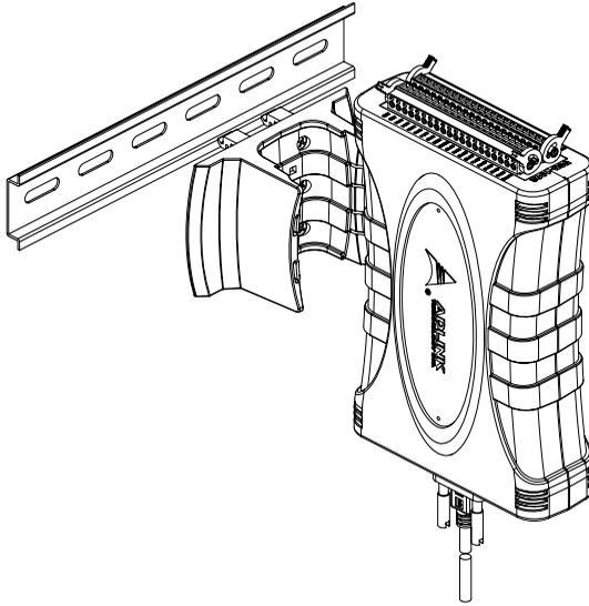
**Figure 2-4: Module Pre-Rail Mounting**
