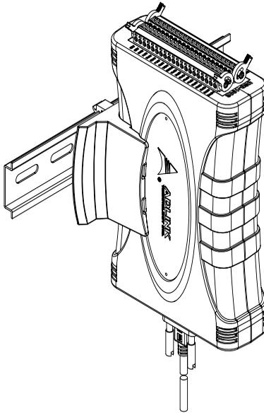
**Figure 2-5: Module Rail-Mounted**
