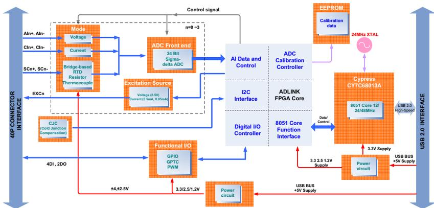
Figure 3-1: USB-2401 Functional Block Diagram
