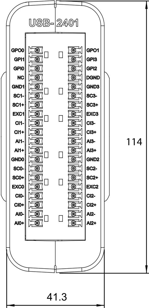
Figure 1-4: USB-2401 Module Front View
