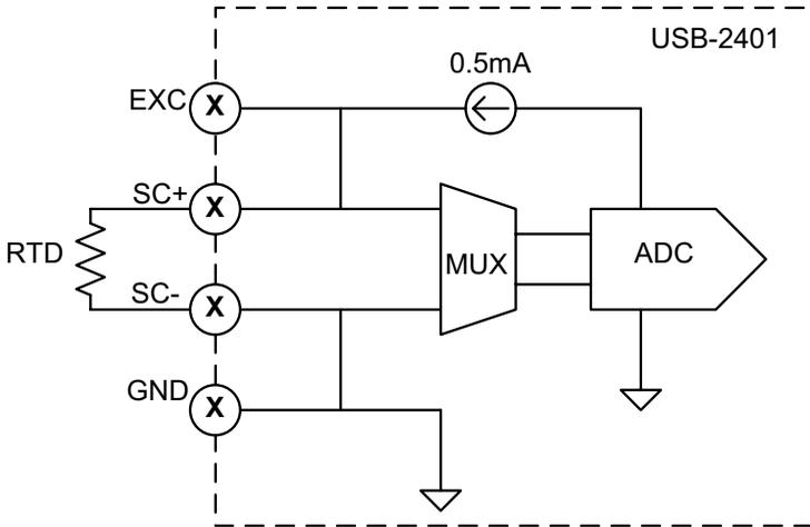
**Figure 3-9: 2-wire RTD Connection**
