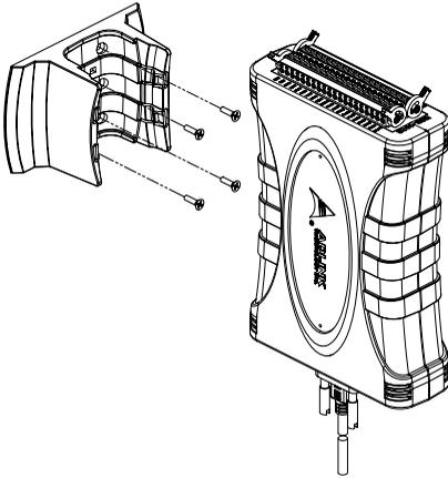
Figure 2-7: Module with Wall Mount Apparatus
