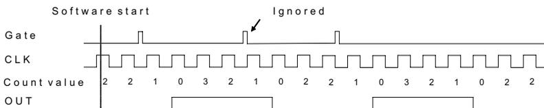
**Figure 3-16: Mode 6-Re-Triggered Single Pulse**
