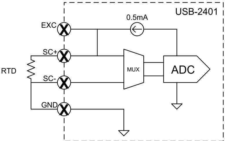
Figure 3-8: 3-Wire RTD Connection
