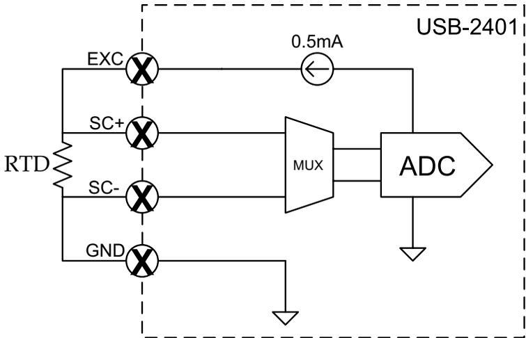
Figure 3-7: 4-Wire RTD Connection
