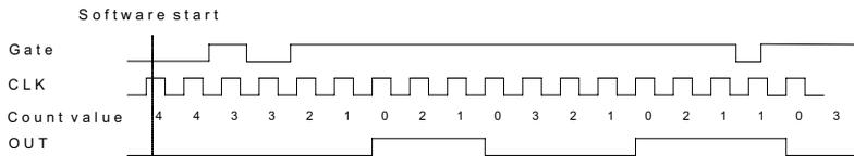
**Figure 3-18: Mode 8-Continuous Gated Pulse**
