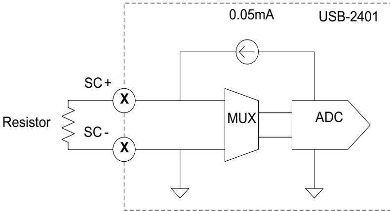
Figure 3-10: 2-Wire Resistance Connection
