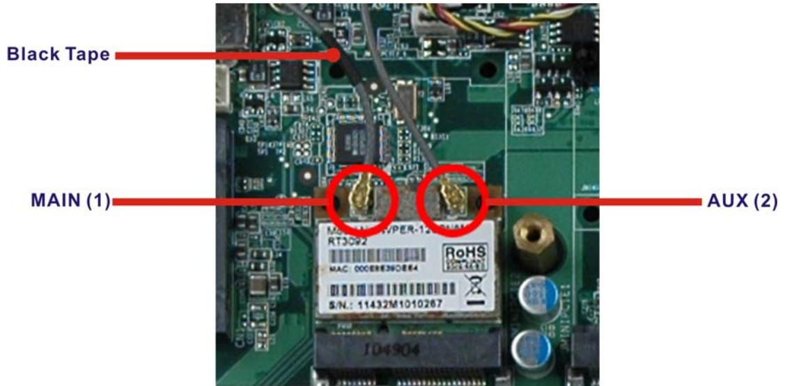
**Figure 5-7: Attaching the Antennas**
