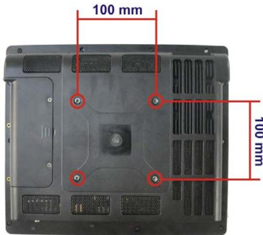
**Figure 4-14: Mounting screw location**
