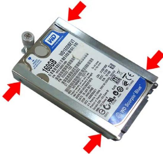
Figure 4-5: Securing the HDD
