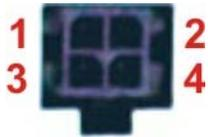
**Figure 4-23: RS-422/485 Serial Port**
