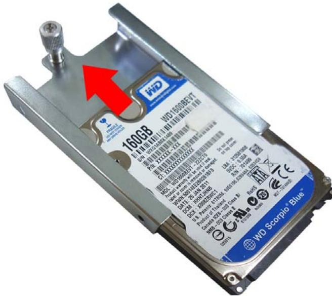
**Figure 4-4: Inserting the HDD**
