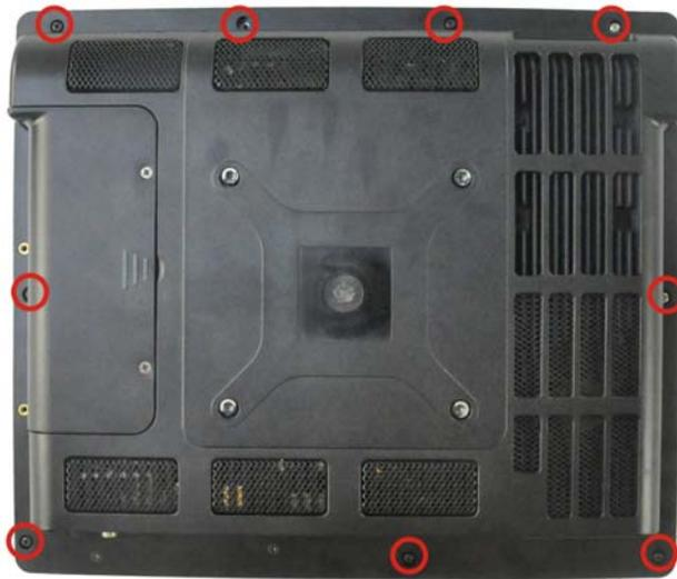
**Figure 5-1: Back Cover Retention Screws**
