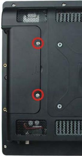
Figure 4-1: HDD Cover Retention Screws
