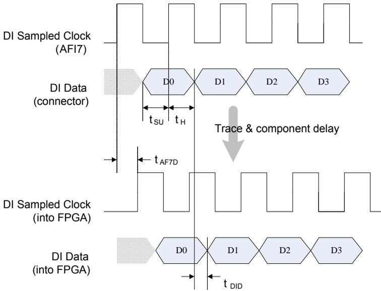
$t_{AF7D}$  = Time delay of external sampled clock from AF17 to internal
