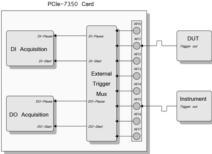
**Figure 3-34: External Digital Trigger Input Configuration**
