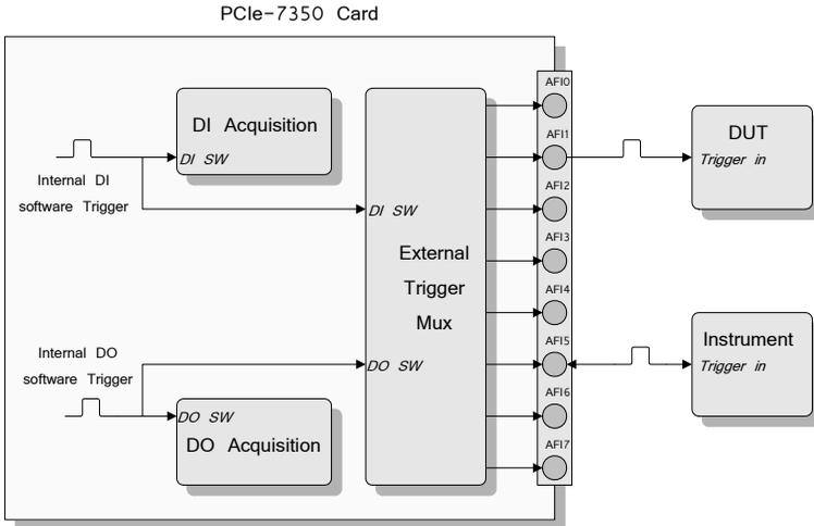
**Figure 3-35: Configured AFI as Internal Software Trigger Output**
