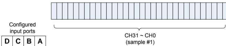
**Figure 3-5: DI Row Data Mapping for 32 Bits Data Width**
