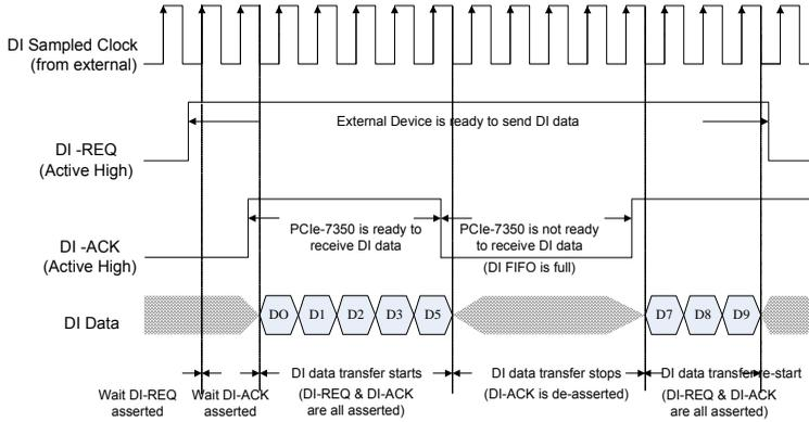
**Figure 3-19: DI Burst Handshaking Timing Diagram**
