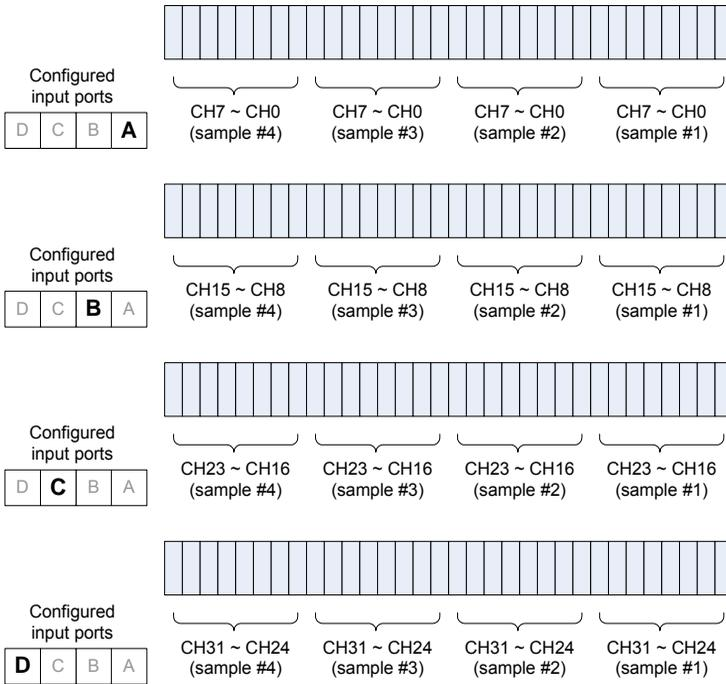
**Figure 3-2: DI Row Data Mapping for 8 Bits Data Width**
