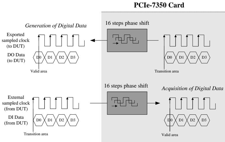
**Figure 3-6: Phase Shift of Sample Clock**
