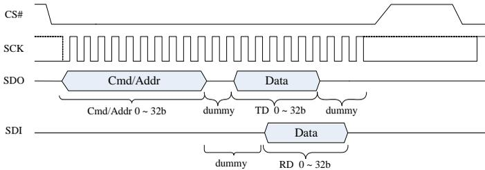
**Figure 3-32: Data Transfer on SPI Bus**
