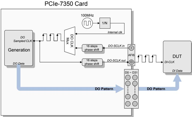
**Figure 3-39: Configured AFI6 as DO Sampled Clock In/Out**
