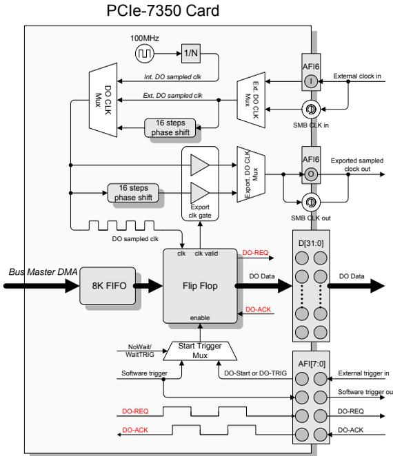
Figure 3-20: DO Burst Handshaking Mode Architecture
