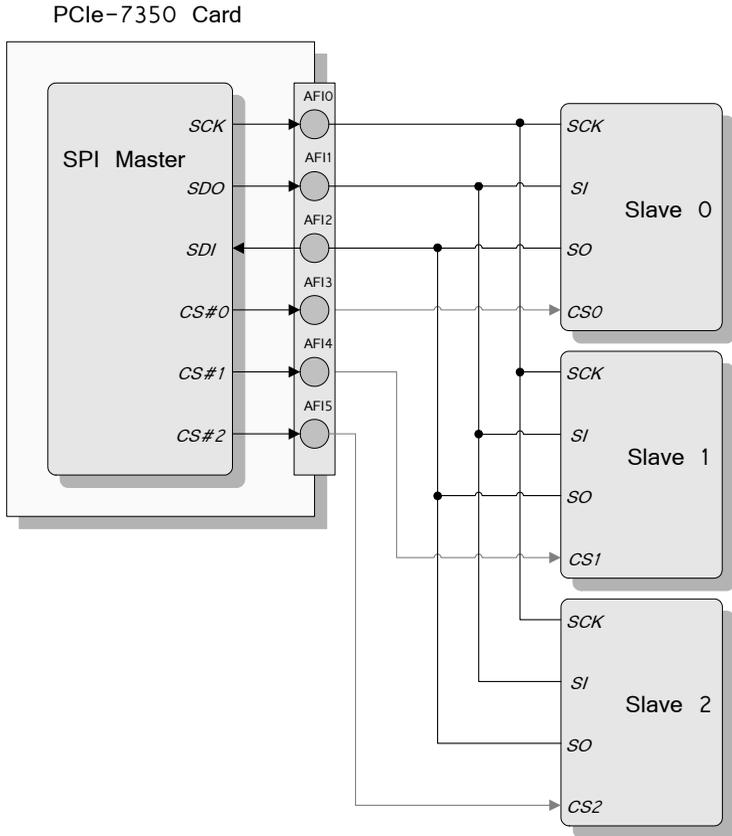
**Figure 3-31: SPI Master of PCIe-7350**
