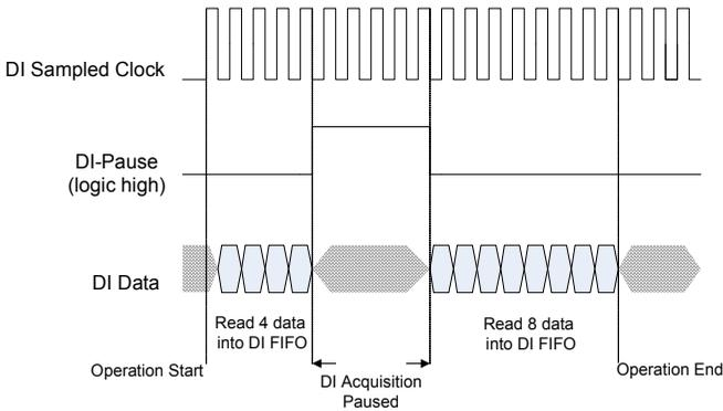
**Figure 3-26: DI Gated Trigger**
