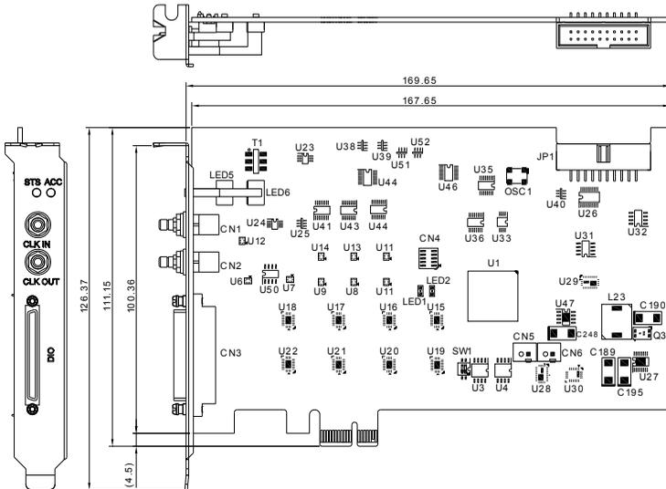
Figure 2-1: PCB Layout and Mechanical Drawing of the PCIe-7350
