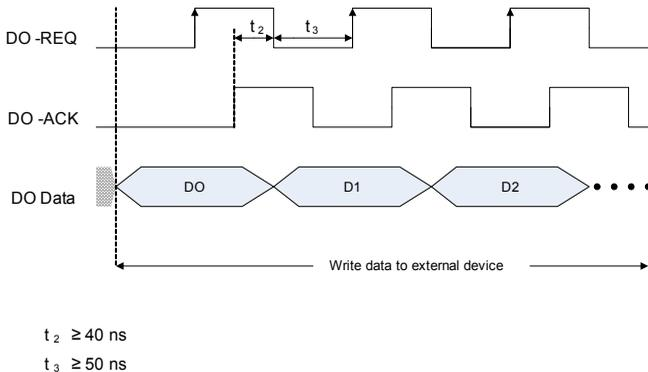
**Figure 3-17: DO Handshaking Timing Diagram**
