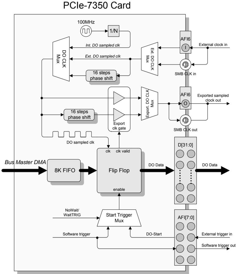
**Figure 3-12: DO Continuous Mode Architecture**
