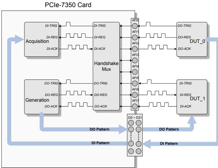
**Figure 3-37: Configured AFI as Handshaking Interface**
