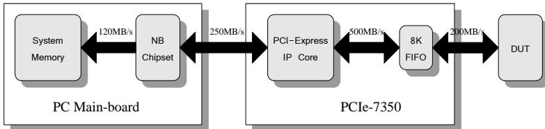
**Figure 3-7: Maximum Data Throughput of the PCIe-7350**
