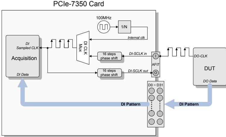
**Figure 3-38: Configured AFI7 as DI Sampled Clock In/Out**
