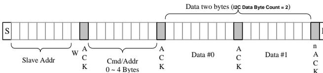
Figure 3-30: I<sup>2</sup>C Data Format
