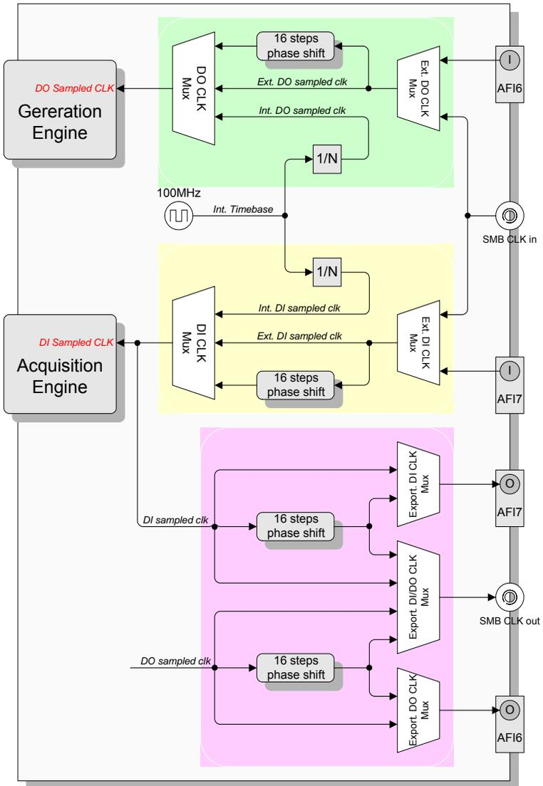
**Figure 3-9: DI/DO Sample Clock Architecture**
