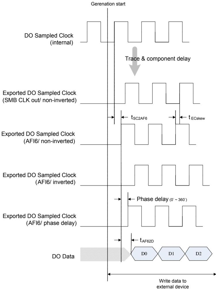
$t_{SC2AF6}$  = Time delay from sampled clock (internal) to exported sampled clock (AFI6)
