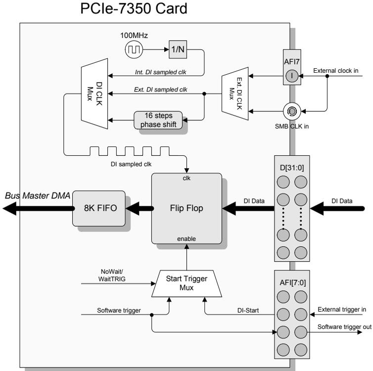
**Figure 3-10: DI Continuous Mode Architecture**
