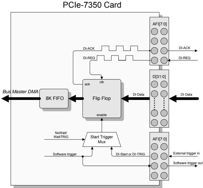
**Figure 3-14: DI Handshaking Mode Architecture**
