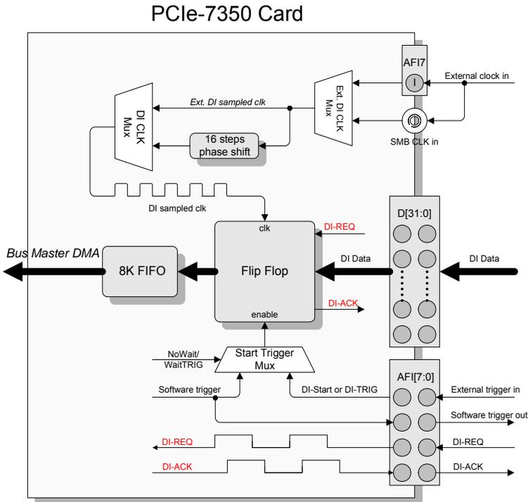
**Figure 3-18: DI Burst Handshaking Mode Architecture**
