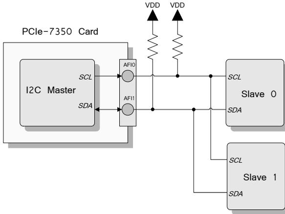
**Figure 3-28: I2C Master of PCIe-7350**
