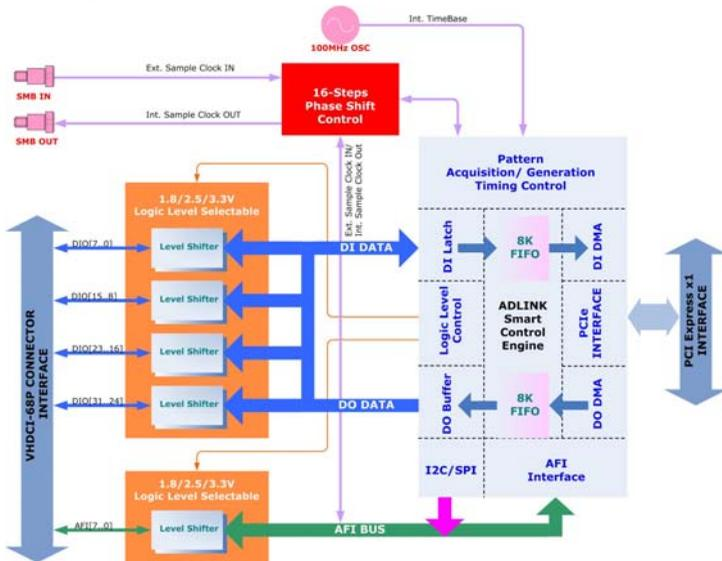
**Figure 3-1: PCIe-7350 Block Diagram**
