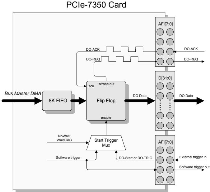
**Figure 3-16: DO Handshaking Mode Architecture**
