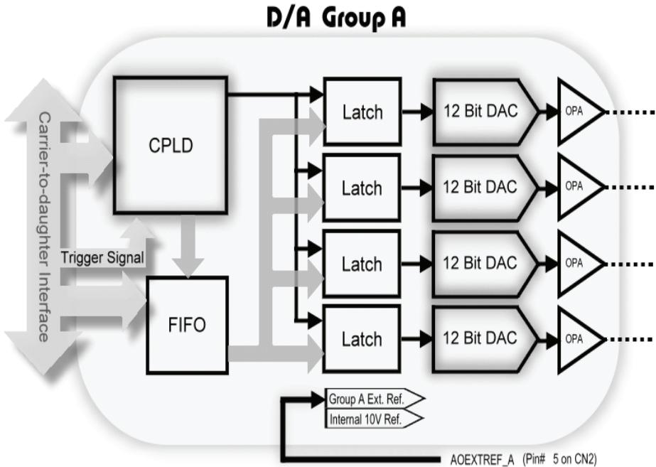
**Figure 4-6: Block Diagram of D/A Group**
