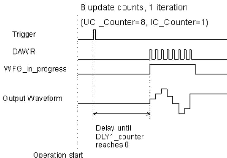
**Figure 4-10: Delay-Trigger Generation**
