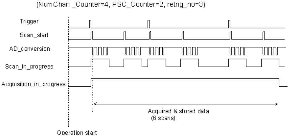
**Figure 4-4: Post trigger with retrigger**
