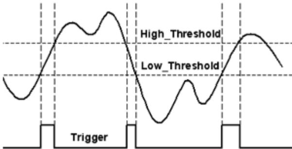
**Figure 4-28: Inside-Region analog trigger condition**
