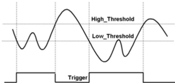
**Figure 4-30: Low-Hysteresis analog trigger condition**
