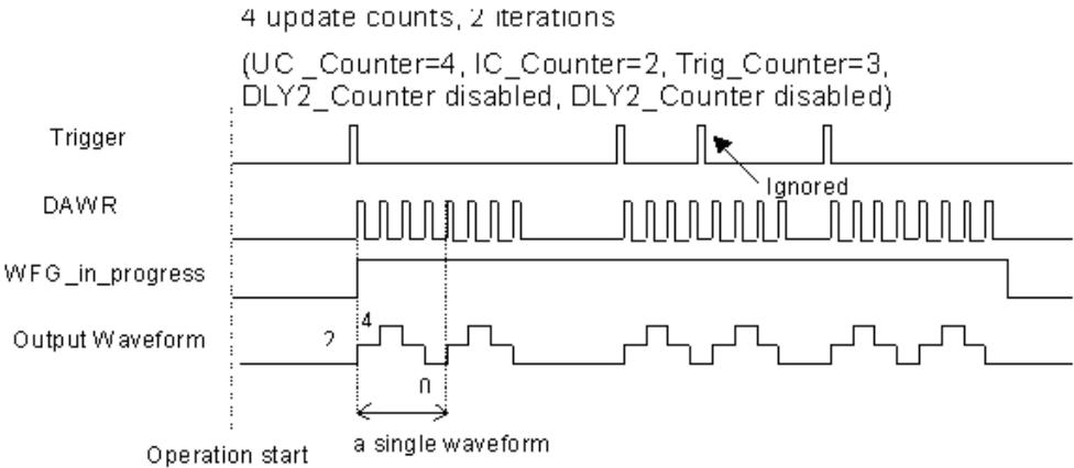
**Figure 4-11: Post-Trigger with Retrigger Generation**
