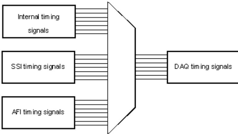
**Figure 4-31: DAQ signals routing**
