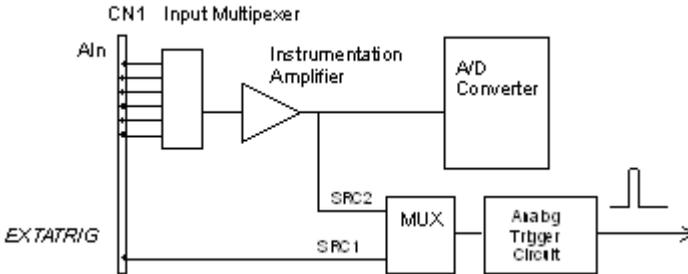
**Figure 4-25: Analog trigger block diagram**
