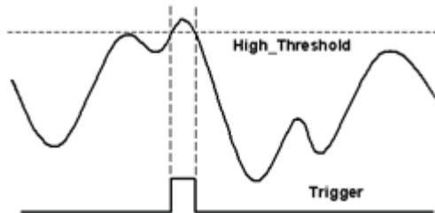
**Figure 4-27: Above-High analog trigger condition**
