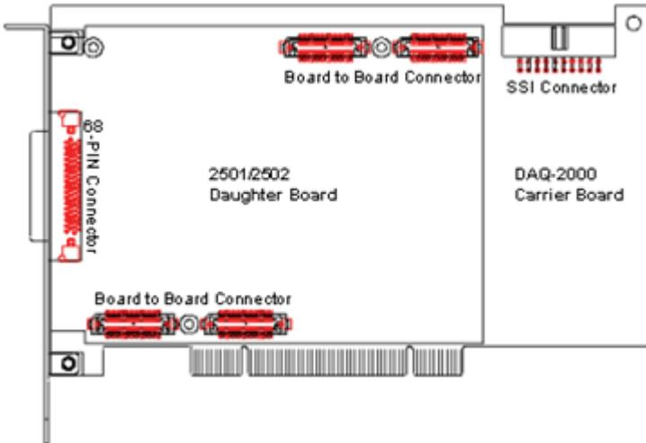
Figure 2-1: PCB Layout of DAQ-2502/2501
