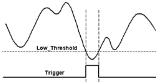
**Figure 4-26: Below-Low analog trigger condition**
