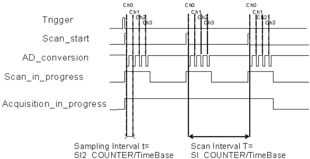
**Figure 4-1: Timing for Scan**
