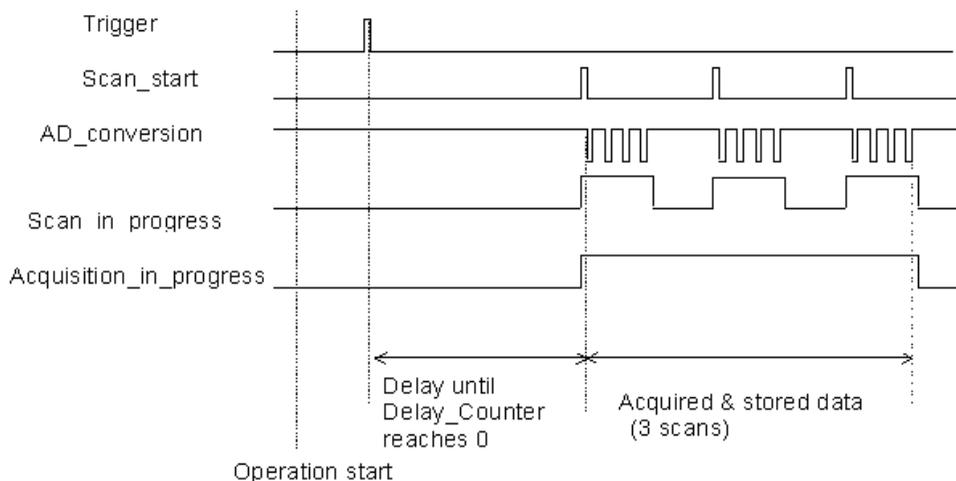
**Figure 4-3: Delay trigger**
