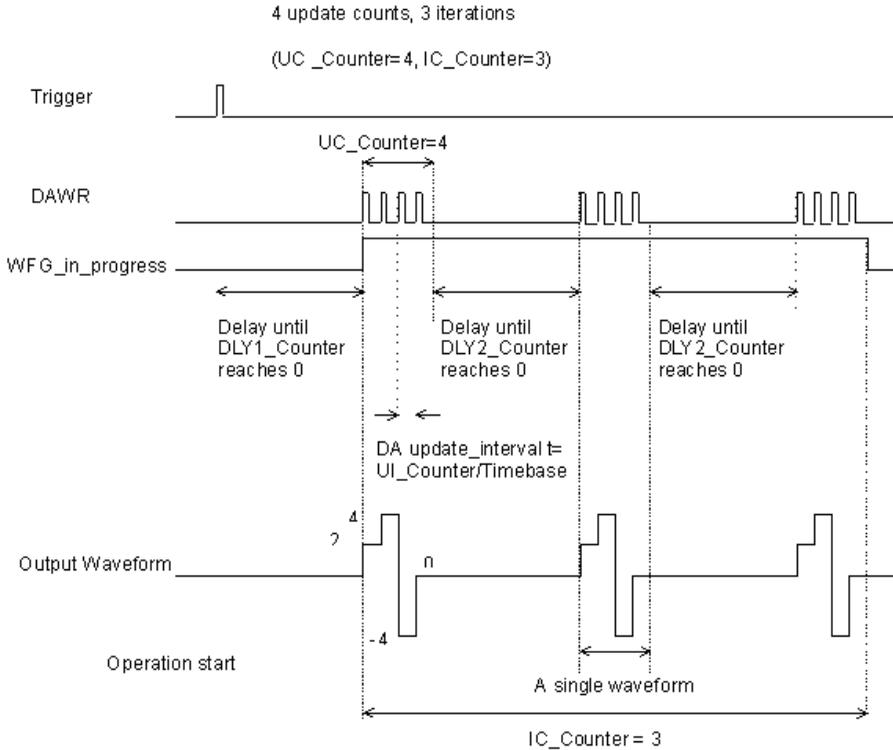
**Figure 4-8: Typical D/A timing of waveform generation**
