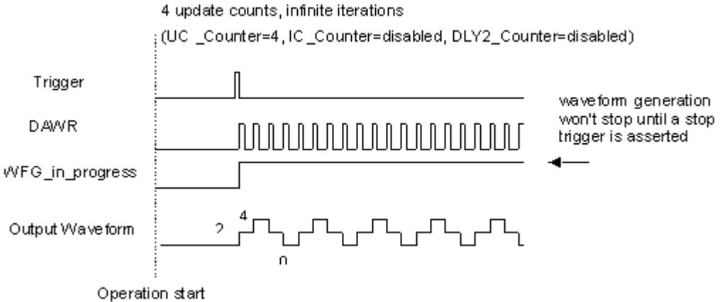
**Figure 4-13: Infinite iterative waveform generation w/Post-trigger**
