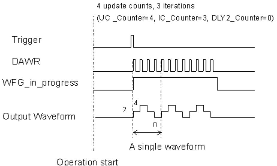
**Figure 4-12: Finite iterative waveform generation w/Post-trigger**
