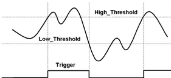
**Figure 4-29: High-Hysteresis analog trigger condition**
