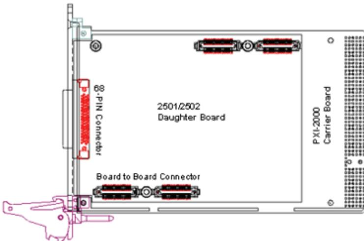
Figure 2-2: PCB Layout of PXI-2502/2501
