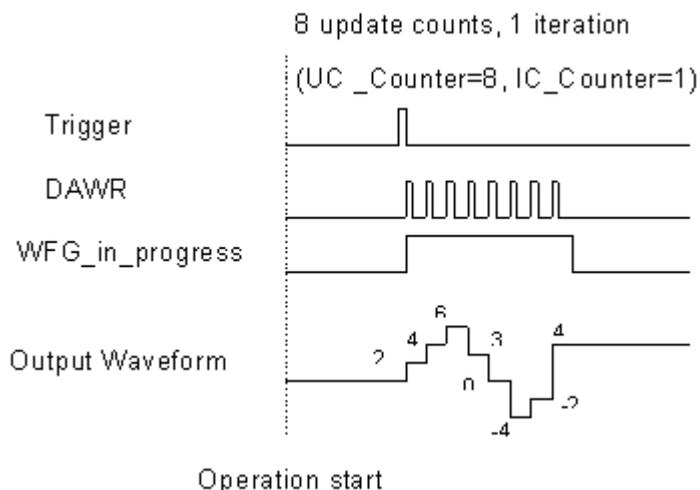
**Figure 4-9: Post-Trigger Generation**
