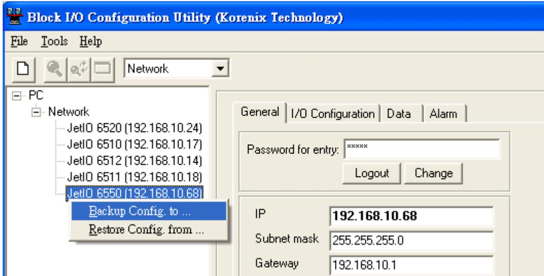
Select “Backup Config. to ...” and “Restore Config. from ...” command to backup and restore the configuration of the JetIO to/from a text file. It should be noticed that you will need to login first and then gain a privilege to do these functions.
