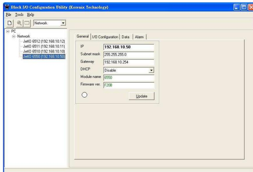
4. Move the mouse over to one of the JetI/O units. Select the unit then you can configure and monitor the configurations of the JetI/O. The features Block I/O Configuration utility provides are similar. Please find your model name and go to its configuration introduction chapter in below.
