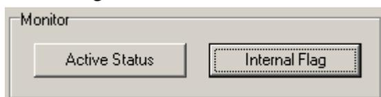
Refer to above Figure as below, in the bottom field of this “Peer to Peer I/O” page is the motoring area. It is monitoring the status both on peer-to-peer I/O activity and internal flags. Click “Active Status” button, the dialog of peer-to-peer I/O active status will popup to represent the status code on peer-to-peer I/O activity.
