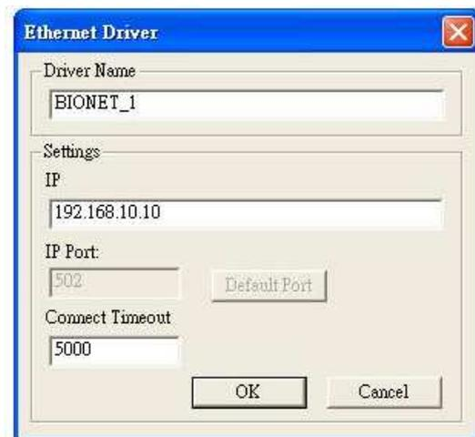
Figure 4.3 "Ethernet Driver" popup Window. Type the Driver Name and IP address for the device.
