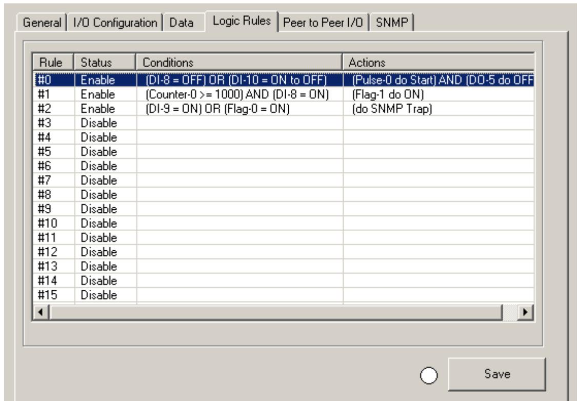
Double click the Rule ID and then you can go to the Logic Rule#ID Configuration page. Select “Enable” and configure the Condition and Actions then press “Apply” to enable the rule.
