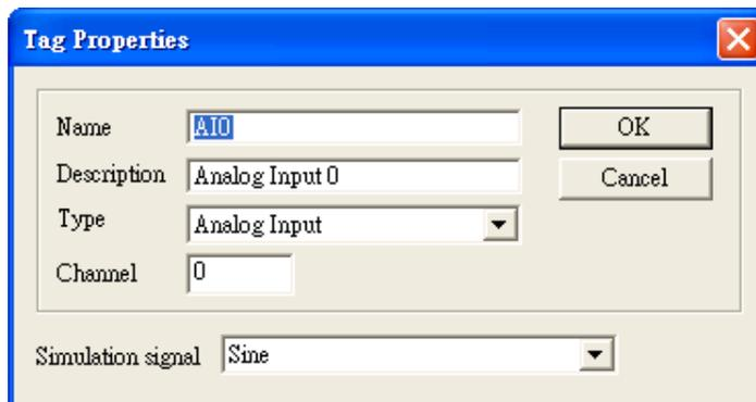
Note: The **Simulation Signal** is used when choosing Simulate I/O mode. Simulate I/O mode is selected in “Device Properties”. This feature allows you to generate simulation values and run testing when you operate the OPC client. You can see the value is continuously changed. The Sine, Ramp and Random are the different type’s simulation signal.
