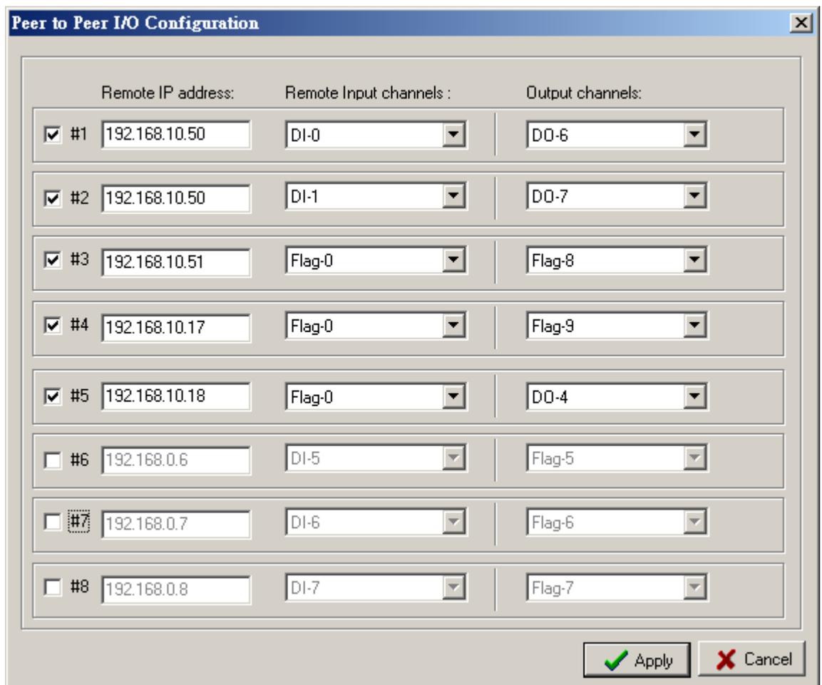
After completing all configurations for Peer-to-Peer I/O activity, click “Save” button, all the mapping configurations will be flushed into flash memory on
