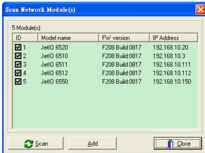
4.1.4.3 Follow the 4.1.4 to practice JetI/O configuration. Select the model and read or write status and configurations. As to how to operate the JetI/O configuration of other model, please refer to its manual.
