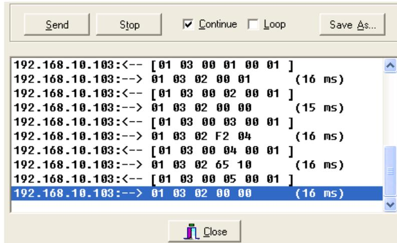
The above screen shows you the result of running “Modbus test.txt” example in 4.1.6.4.
