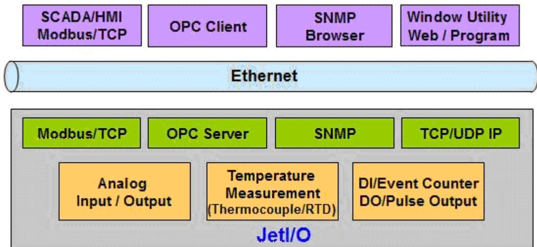
Figure 1. The JetI/O Intelligent Ethernet I/O Server Architecture.
