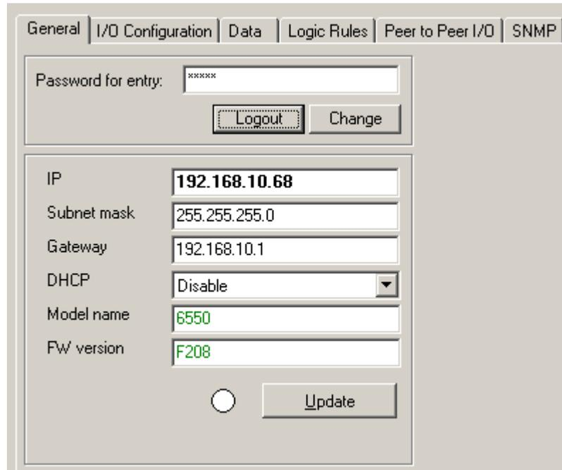
It should be noticed that the privilege setting is required to gain access to do the further configuration options. When you install the I/O module in first time, the default password is “**admin**”. You just need to click on “Login” button and type the password of “Admin” on “password for entry” field. If you want to make password changes, click “Change” button and then the dialog of “Change Password” prompts you to update the new password with up to six characters.
