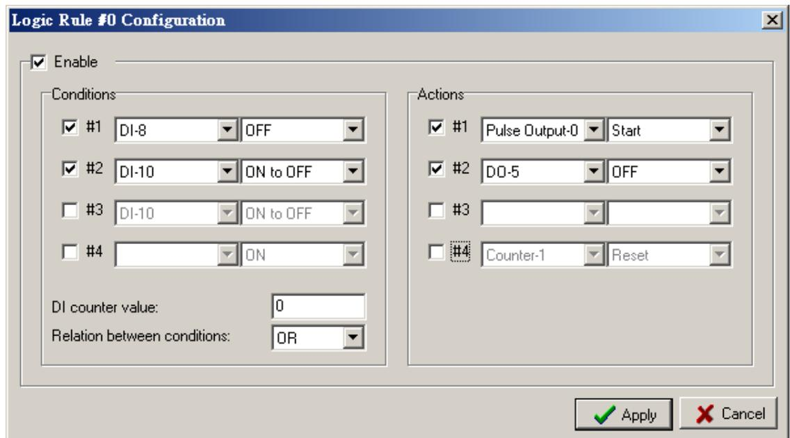
Thus, when the “Conditions” is reached, the system automatically activates the “Actives”. For example:
