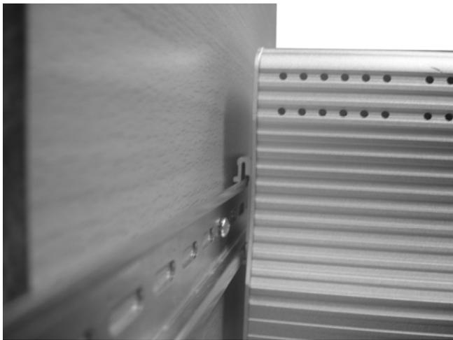
3. Check if the DIN-Rail clip is tightly attached to the track.
