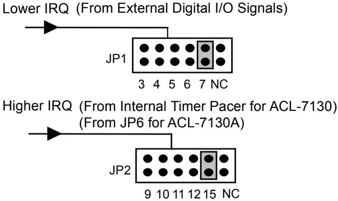
The lower interrupt IRQ can be set as IRQ3~IRQ7 by Jumper JP1. It is illustrated as figure 2.3. The second interrupt IRQ can be set as IRQ9~IRQ15 by jumper JP2. It is illustrated as figure 2.4. Both of lower and higher IRQ can generate interrupt simultaneously.
