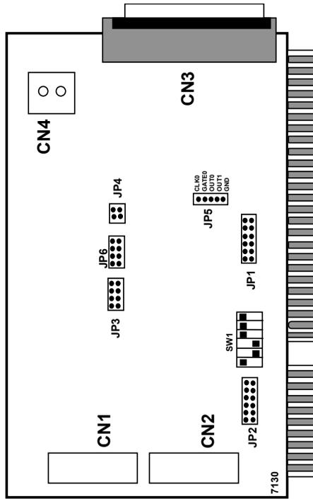
Figure 2.1 PCB Layout
