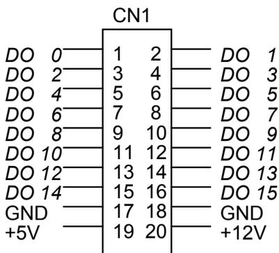
**Figure 2.9 Pin assignment of Connector CN1**
