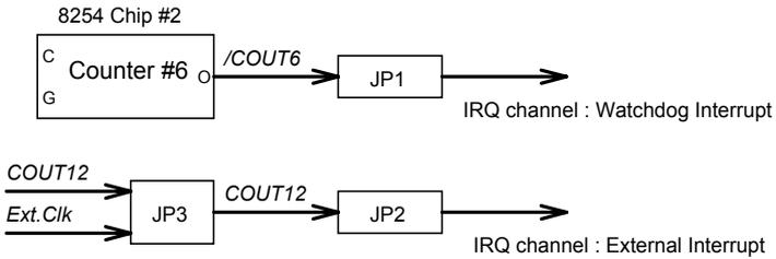
Figure 4.8 Example of double interrupt system
