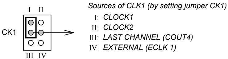
**Figure 2.13 Setting the Clock Source of Counter #1**
