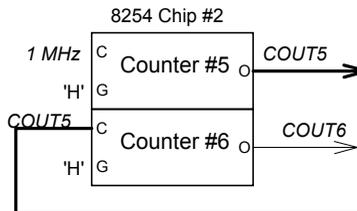
Figure 2.10 Example of 'cascaded counter'
