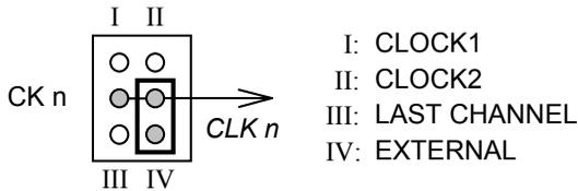
The Table 2.4 shows the reference number of the clock source jumpers and its corresponding counter/timer channels number. The default setting of every jumper is also shown. The clock sources of **CLK1~4** come from internal source '**CLOCK1**' and the clock sources of **CLK7~10** come from external sources.
