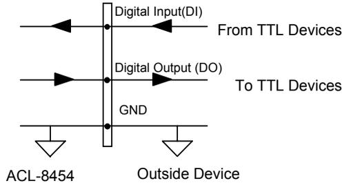
**Figure 4.1 Digital I/O Connections**
