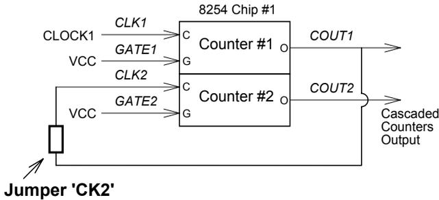
Figure 2.11 Example of 'user configurable cascaded counters'
